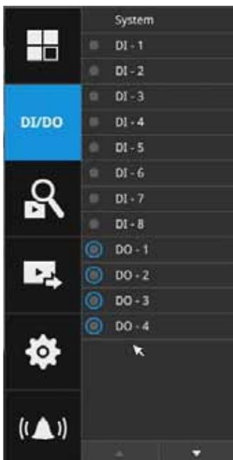
Click on the DI/DO button to display the system's DI and DO signals (whether they are connected or not). If a digital input signal is triggered, e.g., the DI-4 on the left, its indicator will turn solid white.
