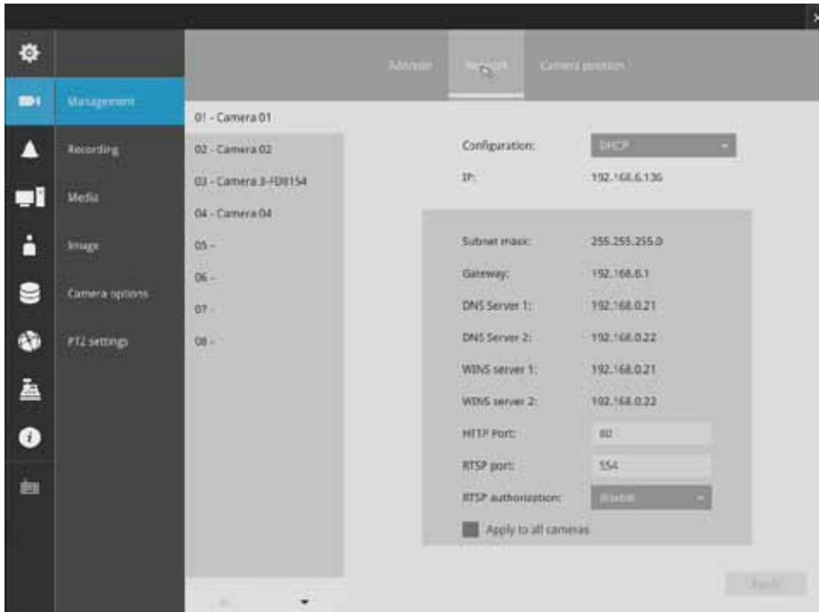
You can select DHCP as the method for cameras to acquire IP addresses, or you can manually configure static IPs for a single or all cameras. Using static IPs is recommended. Although the NVR can remember the MAC addresses of cameras, if IPs are changed under the DHCP configuration, your NVR may still fail to connect the cameras. Please consult your network administrator for details about network settings.
