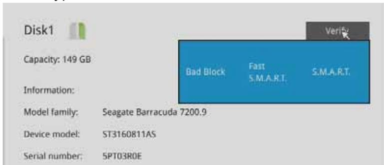
**Bad block check:** Performs read/write test to drive sectors to locate bad blocks. This action may take several hours to complete.
