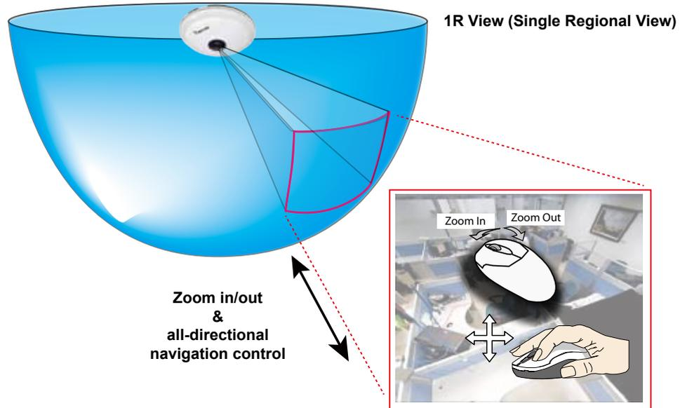
The 1R mode (or rectilinear) provides access to one image section within the hemisphere. You can zoom in or out (using the mouse wheel or PTZ panel) or travel through to other areas within the hemisphere using simple mouse clicks and drags. A single click on a particular object can bring the object to the center of your view window. Click and hold down the left mouse button, and you can swipe the view both horizontally and vertically.
