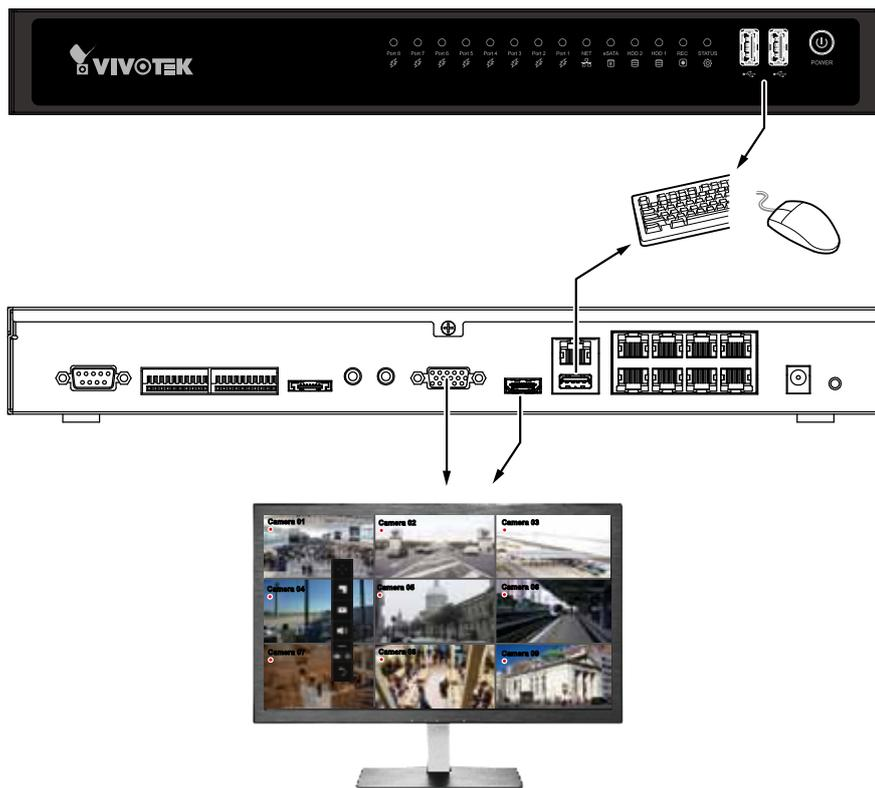
By default, a live view appears on an HDMI monitor. The interface architecture of the local console is illustrated as follows:
